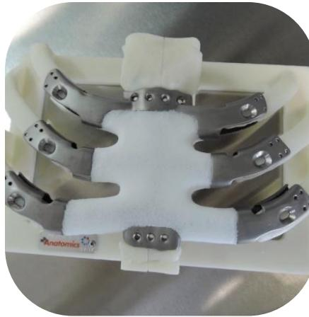
The team at the metal 3D printing facilities at the Commonwealth Scientific and Industrial Research Organisation (CSIRO) used electron beam melting method to build up layers of titanium powder and melt them together to print the implant based on the patient's CT scans.<sup>180</sup>
