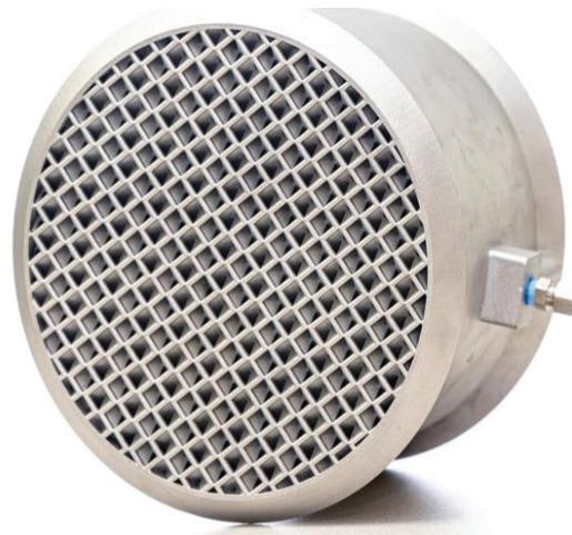
The team tested the novel circular device, which integrates a heat exchanger with a mass-exchanging contactor (Figure 6). The researchers conducted a series of experiments to determine which
